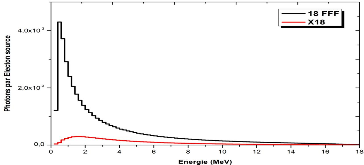
Calculated photon energy Spectra at the isocentre for the 18 MV flattened and unflattened photon beams, over 10 x 10 cm<sup>2</sup> field size
