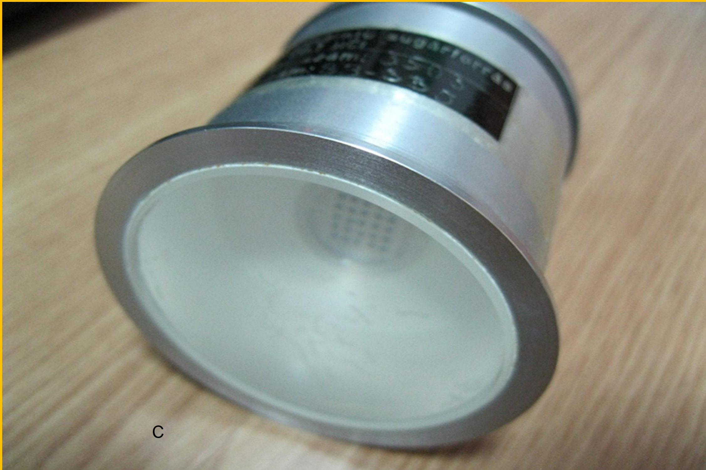
NaI(Tl) scintillation crystal sealed in dural with Am-241 embedded in crystal
