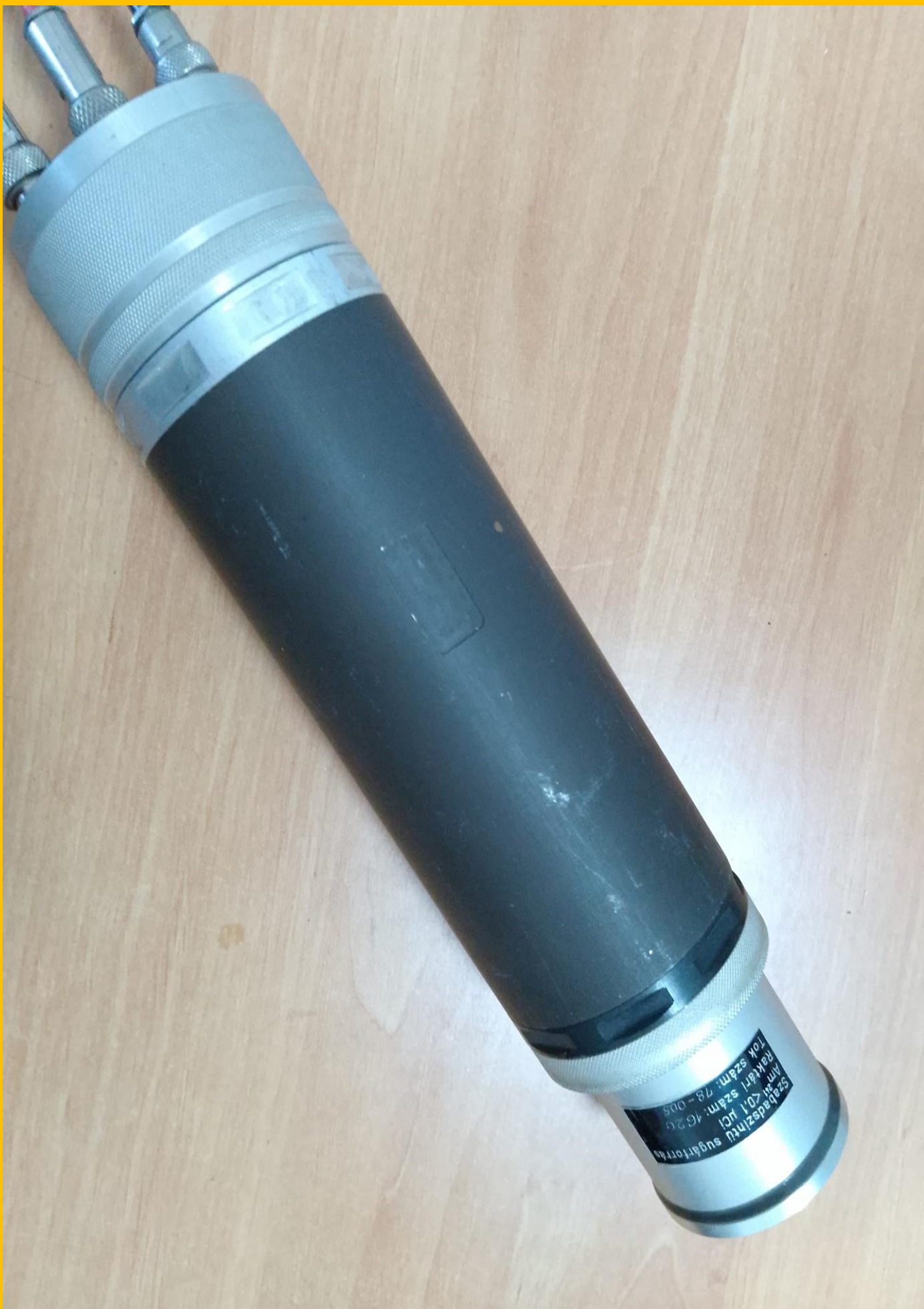
Scintillation probe of NaI(Tl) with photomultiplier readout
