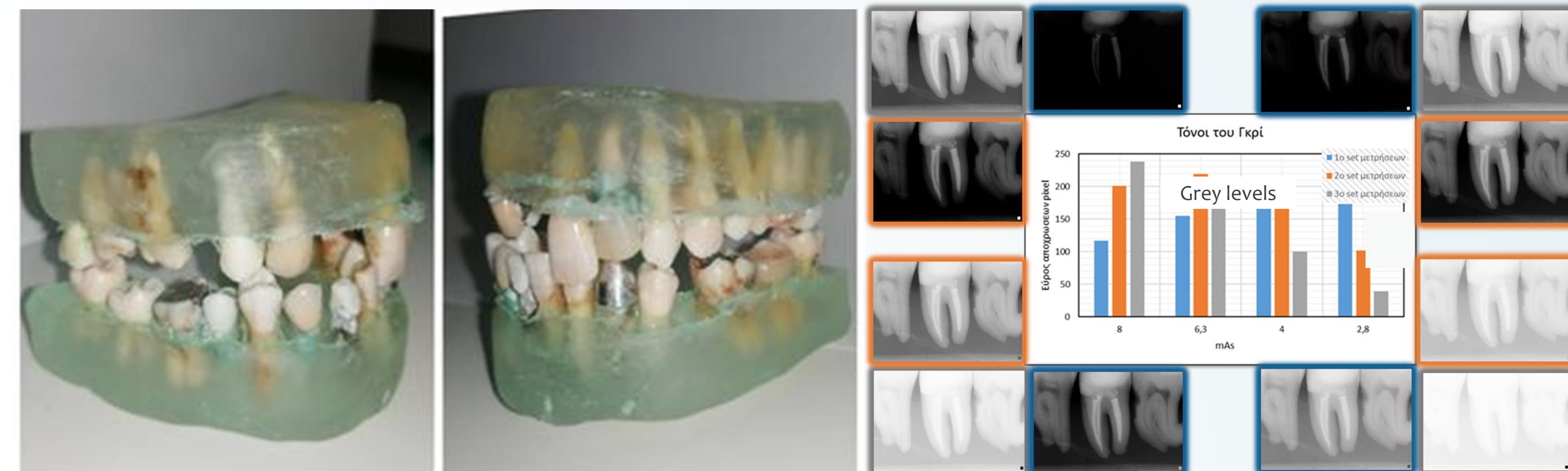
Figure 5. The final result of the phantom. Periscopic views of the rear part of the phantom and diagram - range of grey levels.
