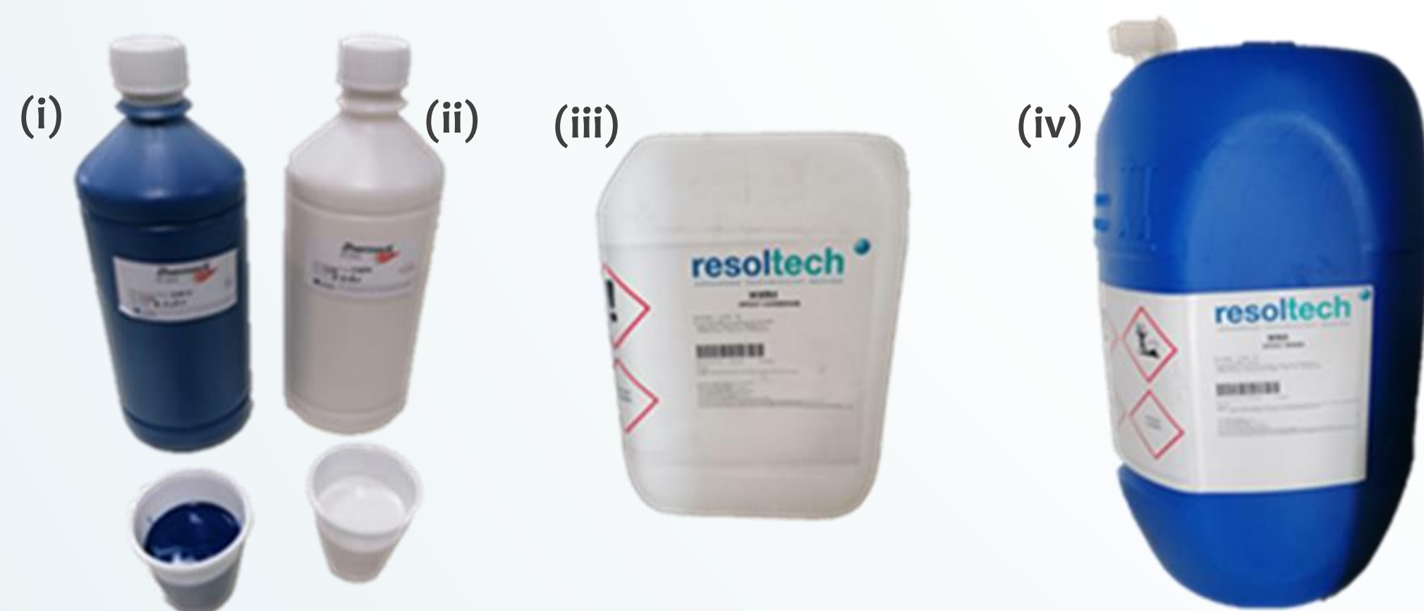
Figure 3. Materials for the manufacture of female silicone molds for the jaw shape creation and the resin for the simulation of the soft tissue X-ray attenuation. (i) Base of the silicone, (ii) catalyst for the hardening of silicone, (iii) WWB4 EPOXY HARDENER, (iv) WWA EPOXY RESIN.
