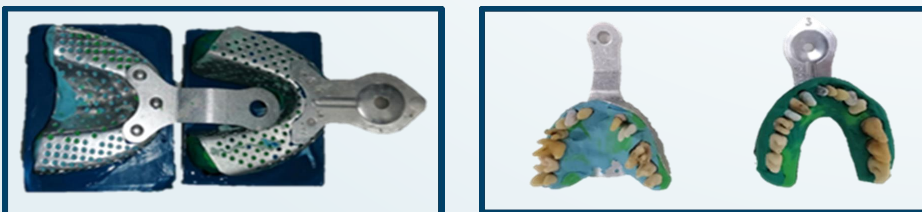
Figure 4. Image on the left: Iron molds that served to obtain both jaw imprints and plasticine for the teeth integration within the resin. Image on the right: Female molds with epoxy resin inside them and the molds placed on top to immerse the roots of the teeth.
