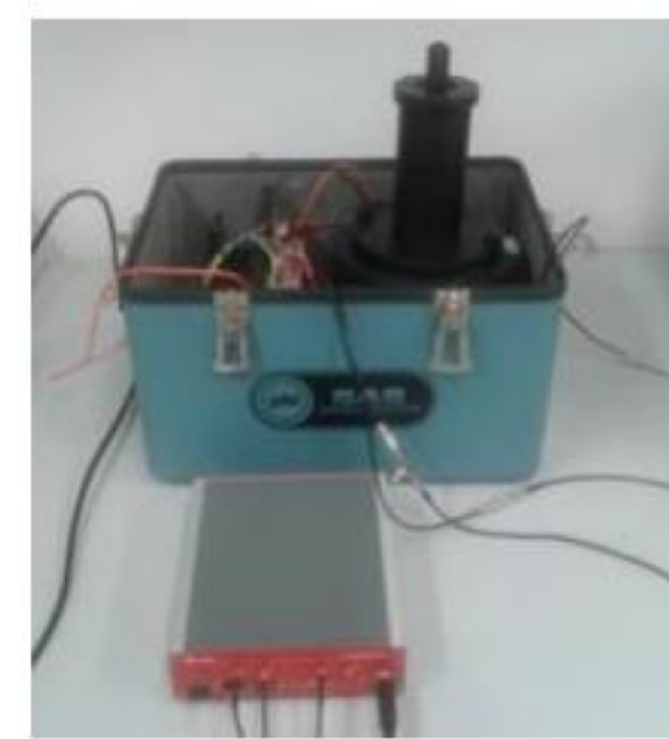
Fig.2: Blue box contains the TDCR system, the power supply and the digitizer. It is covered, during measurements, to avoid the enter of light in the system and there is only a little hole for placing the vial. The portable TDCR is connected to the alimentation system and to the digitizer. The latter processes the pulses from the detector, recording the signal arrival time and signal amplitude in an external file. These signals are off-line analyzed by a software implemented in CERN ROOT frame and developed at ENEA-INMRI.
